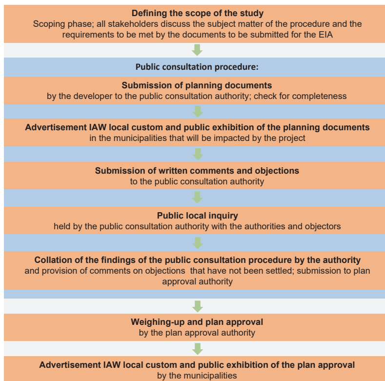
Fig. 8: Flow chart illustrating a plan approval procedure with EIA
